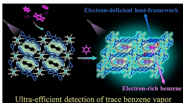
Figure 27 (Color online) Schematic for detection of trace benzene vapor by WYU-61. Reproduced with permission from Ref. [296]. Copyright©2023, Wiley-VCH GmbH.
